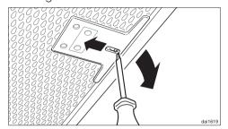
If the filters are incorrectly installed, insert a small screwdriver into the slit along its edge to disengage them from the casing.
